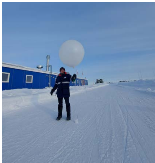
Fig. 7: Another part of the daily work is the ascent of radiosondes to obtain a profile of the current state of the atmosphere (Photo: Michael Schäfer).
